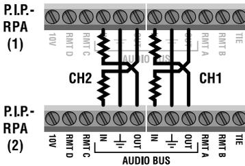
Fig. 3.17 Stacking Two P.I.P.-RPAs
