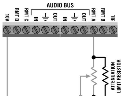
Fig. A.3 Adding an Attenuation Limit Resistor Parallel to the Remote Pot
