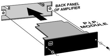
Fig. 3.9 Installation into a Standard PIP Amplifier
