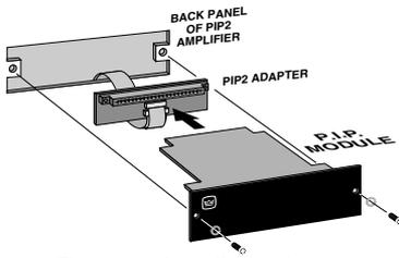
Fig. 3.11 Installation into a PIP2 Amplifier
