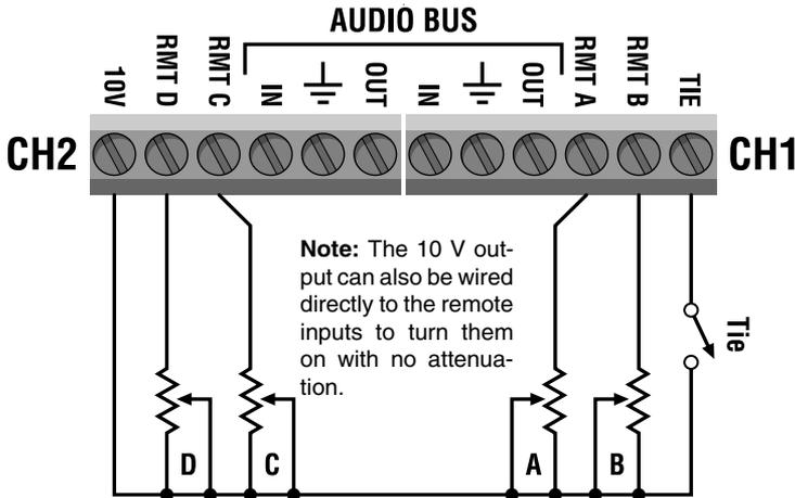
*Fig. 3.16 Remote Control & Tie Function Wiring*
