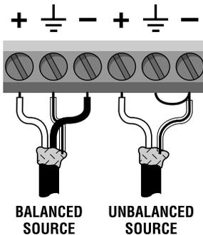
Fig. 3.12 Main Audio Input Wiring
