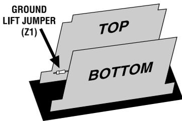
Fig. 3.13 Locating the Ground Isolation Jumper
