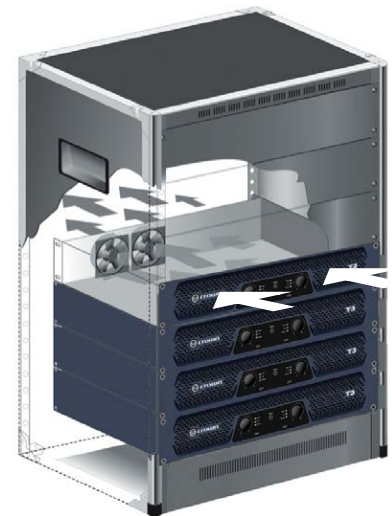
Figure 2: Proper rack venting
