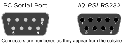
Connectors are numbered as they appear from the outside.
