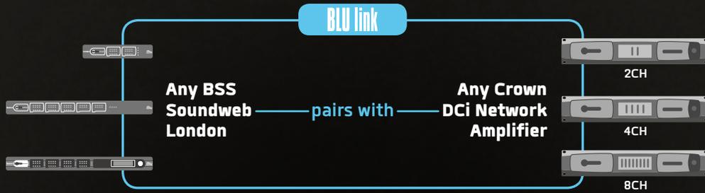
BLU link is not only a standalone audio transport, it's complementary! To save on costs and add convenience, run AVB, CobraNet, or Dante through a BSS Soundweb London and convert audio to BLU link. BLU link enables an easy and flexible range of audio solutions through its increasing presence in HARMAN products.
