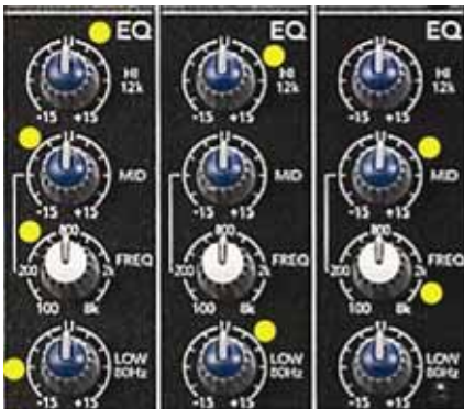
Figure 2. Marking EQ settings with adhesive dots.
