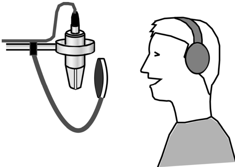
Figure 4. A large-diaphragm cardioid condenser mic with a pop filter and shock mount.
