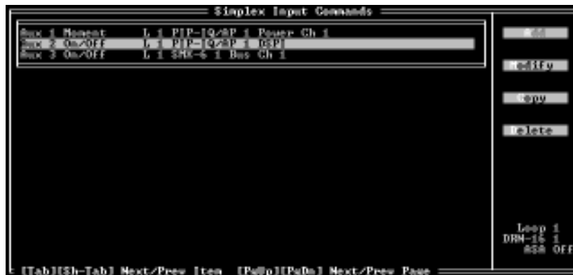
Fig. 8.7 Selecting an Existing Drone Command Assignment
