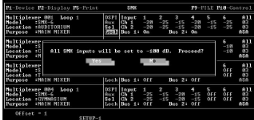
Fig. 6.7 Turning the SMX-6 Lock Feature On Sets All Gain Controls to -100 dB
