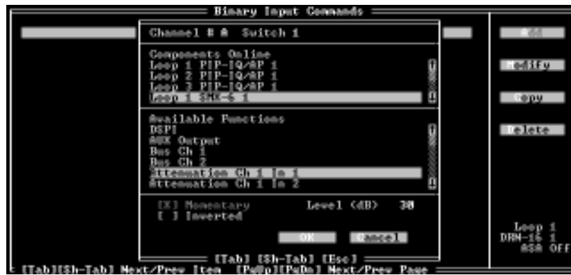
Fig. 8.8 Adding a Command Assignment to a Binary AUX Input
