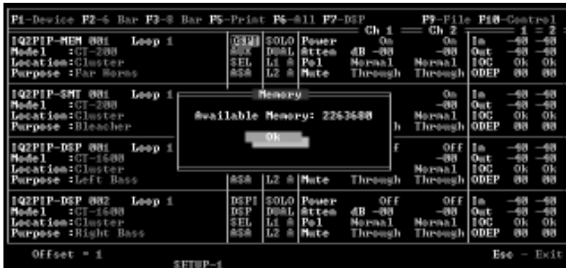
Fig. 2.29 Checking Available Memory from a Control Block Screen
