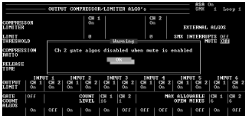
Fig. 6.16 Turning On the Mute Function Will Disable the Gate Count Function for Channel 2
