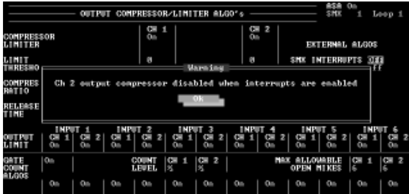
Fig. 6.15 Turning On the SMX Interrupts Function Will Disable the Output Compressor/Limiter Function for Channel 2
